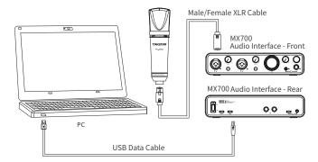
2 Connection to audio device without built-in 48V phantom power:
